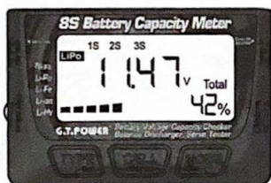
Total voltage and capacity of Lithium Battery
