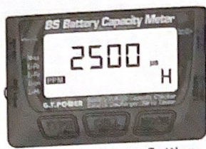
Servo Test Range Setting Servo Test Signal Range setting: 500-2500us
