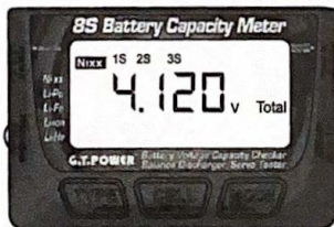
Total voltage and capacity of Nickel battery
